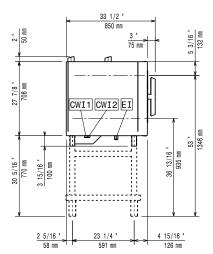
Cold Water inlet 1 (cleaning) Cold Water Inlet 2 (steam CWII CWI2
